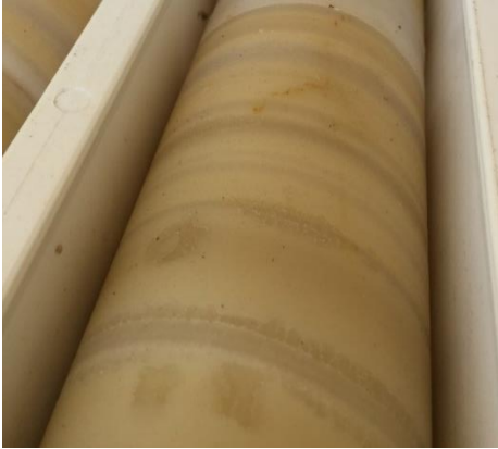
Photo: Colluli kainite core Colluli salts will be mined in solid form
